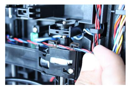
**d** Loop the cable behind the right cable holder.
