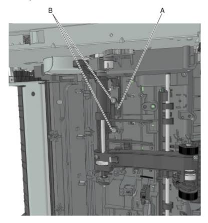
**b** Apply RheoGel 793 to the point of contact between the bracket (A) and cam.
