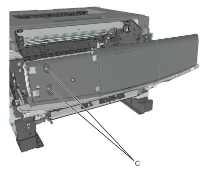
**8** Route all cables off the printer to completely remove the control panel assembly.
