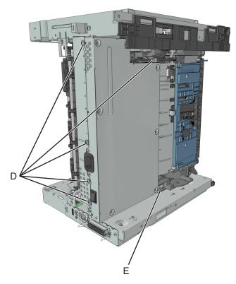
**7** Remove the power supply, and then disconnect all cables from the power supply.
