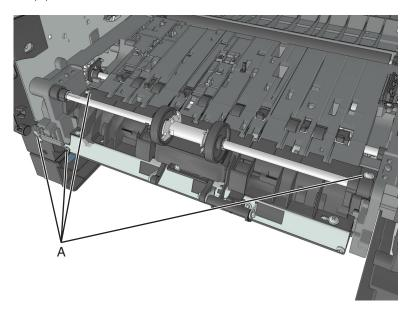
**8** Push and hold the cam restraint to release the MPF shaft.
