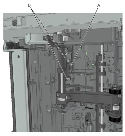
**9** Disconnect the cable from the sensor.
