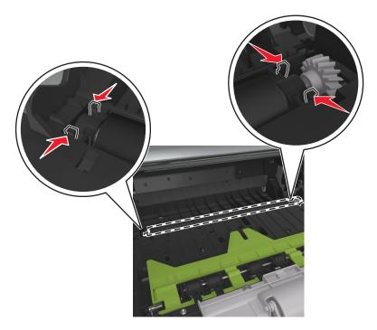
**2** Lift to remove the transfer roll.
