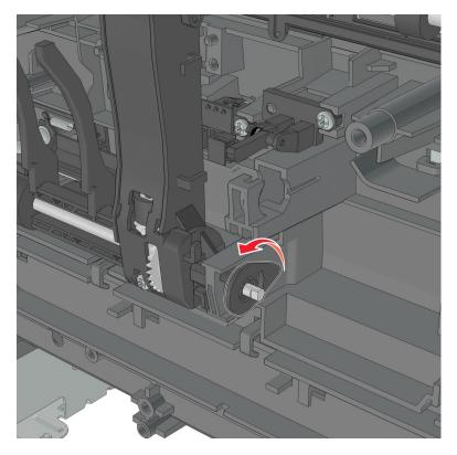
**16** Pull out the shaft, and remove the ACM.
