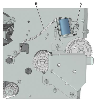
**6** Remove the other half of the cable from the printer.
