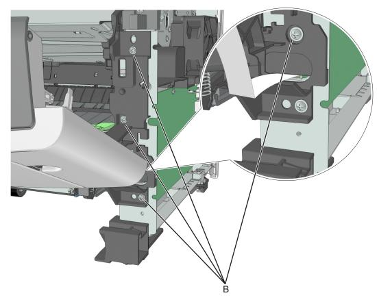
**7** Remove the right front mount, and then remove the front door. Below are the front door and the right front mount.
