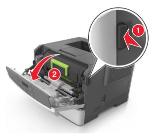
**2** Pull the toner cartridge out using the handle.
